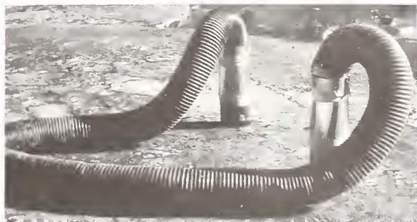
FIGURE 7.—Fan unit and external connections between the aeration ducts at the base of the tanks.
